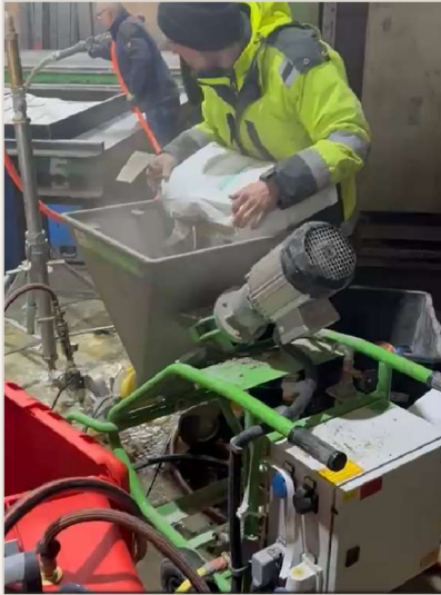
I-FOAM WITH PLANT MACHINE + FOAM GENERATOR
