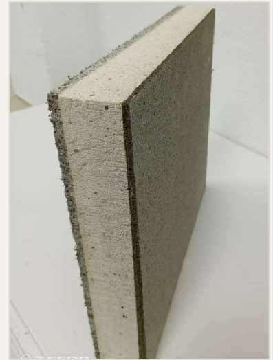
I-FOAM AS AN INSULATION CORE
